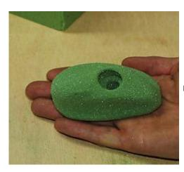
Now your foam mold is ready to be applied into the casting phase of making your custom handhold!
