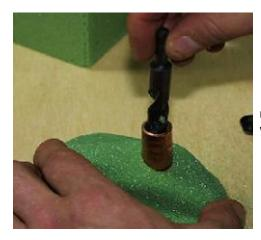
Using the drill bit and a little tube to guid it, drill out the hole for your bolt. Then, using a larger drill bit, widen the top part of the hole so that a bolt head and rachet socket will be able to fit in there.
