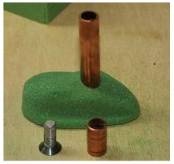
It's time to bore out a hole in your foam so that a bolt or screw will be able to go through your final mold project. You will need a couple different sized drill bits, and the bolts that you're going to use to fasten your handholds to make sure they're going to fit.
