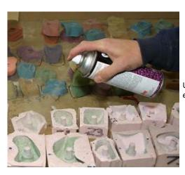
Using Stoner Urethane Mold Release, spray the inside of all the molds to achieve maximum mold life expectency.
