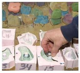
Place washers in the molds. These will help displace the compression from the bolt to prevent overtightening and breaking thin or small holds.
